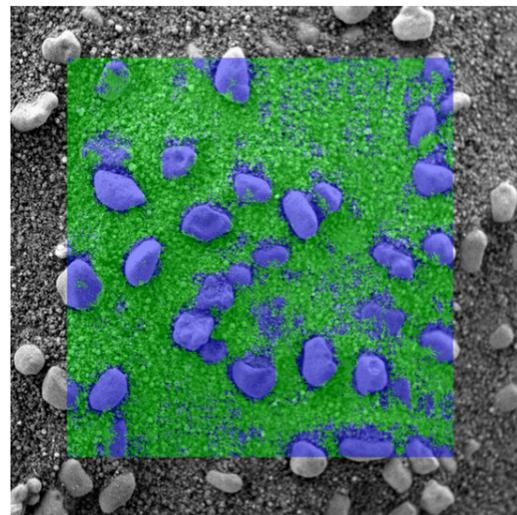
Figure 1. Automatic inference of particle sizes in MI images. Here the system identifies areas where particle sizes are predominantly large sand (blue) and medium sand (green). Image scale: approximately 10cm.
