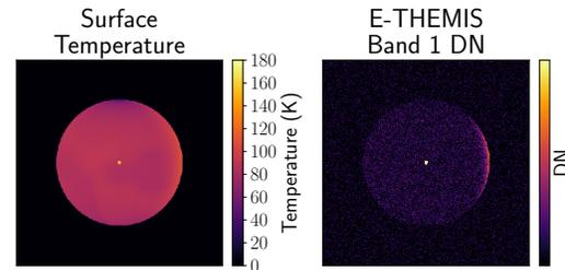
**Figure 1:** An example simulated E-THEMIS observation showing the instrument field-of-view in both temperature and derived DN values for Band 1 (7–14  $\mu\text{m}$ ).
