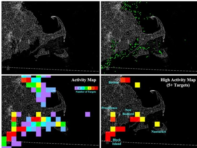
**Fig. 4.** (Top Left) MISR nadir view of Cape Cod, 1 September 2009. (Top Right) Moving ships identified through manual inspection of MISR imagery. (Bottom Left) Corresponding activity map summarizing vehicle activity. (Bottom Right) Summary map of highest vehicle activity (defined as more than 5 targets per region).
