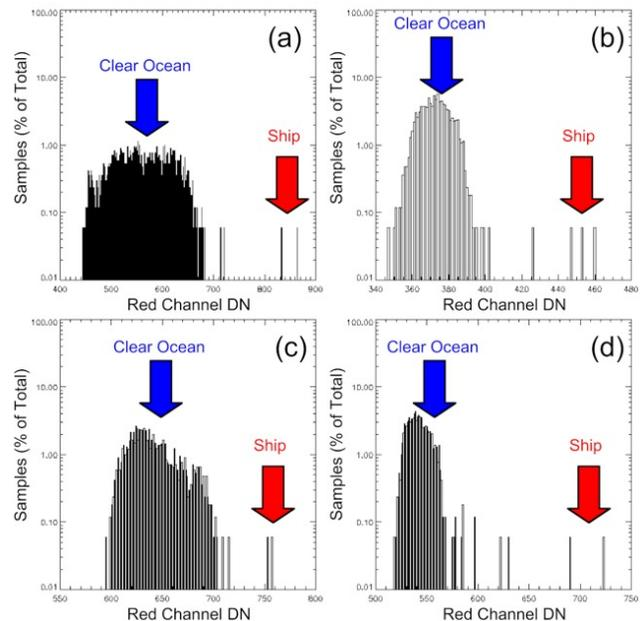
**Fig. 2.** Histograms of MISR red band digital numbers (DNs) for scenes displayed in Fig. 1. The SNR in decibels ( $SNR_{dB}$ ) is calculated by multiplying the log base 10 of the SNR by 20. Most values belong to clear ocean (low DN), with high values corresponding to ships. (a)  $SNR=5$ ,  $SNR_{dB}=13.9$ ; (b)  $SNR=10$ ,  $SNR_{dB}=20.4$ ; (c)  $SNR=7$ ,  $SNR_{dB}=16.5$ ; (d)  $SNR=18$ ,  $SNR_{dB}=24.9$ .
