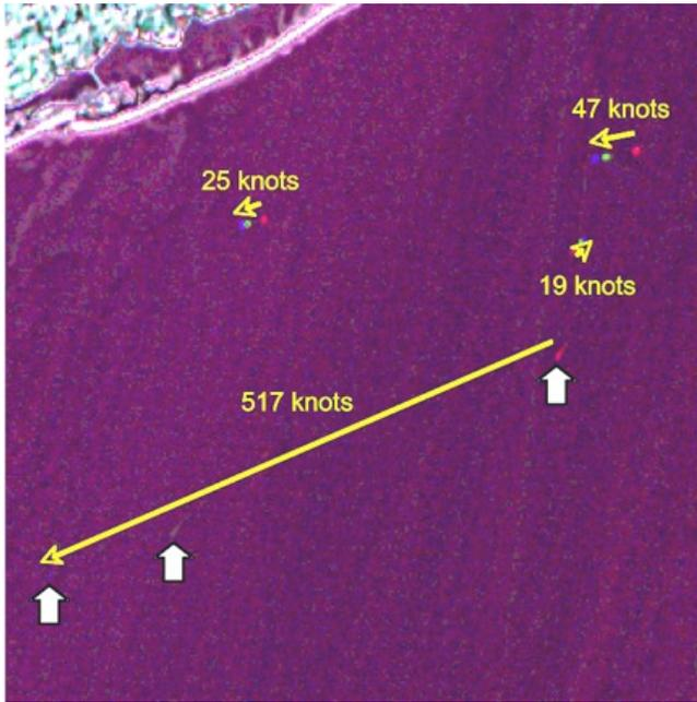
**Fig. 3.** Multiangle color composite [ $+70^\circ$  (red),  $-46^\circ$  (green),  $-70^\circ$  (blue)] from MISR images (17 April 2008) enhanced by the application of a bilateral filter. Long Island, NY, is at the upper edge of the image. Moving targets appear as sequences of red, green, and blue points. Yellow arrows (short = ship, long = airplane) indicate manually derived trajectories (speed and direction).
