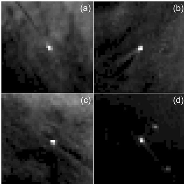
**Fig. 1.** Four examples of ships in dynamically stretched MISR data showing the multi-pixel features they generate: (a) Red Sea, 2 April 2003; (b) Atlantic coast off Long Island, NY, 1 April 2008; (c) Strait of Malacca, 18 August 2009; (d) three ships, Gulf of Oman, 24 February 2010.
