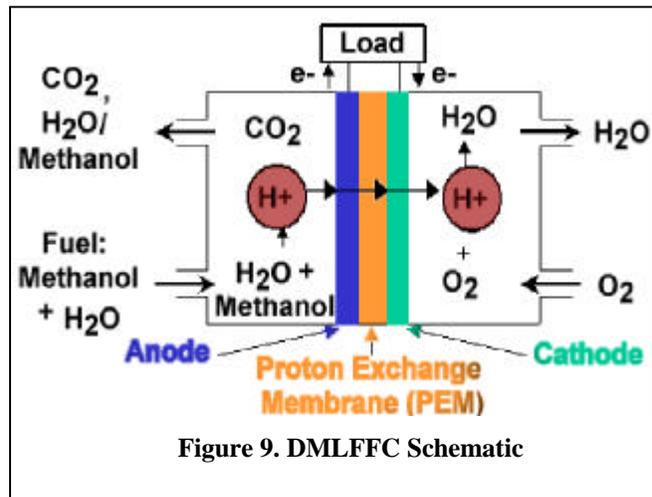
Figure 9. DMLFFC Schematic
