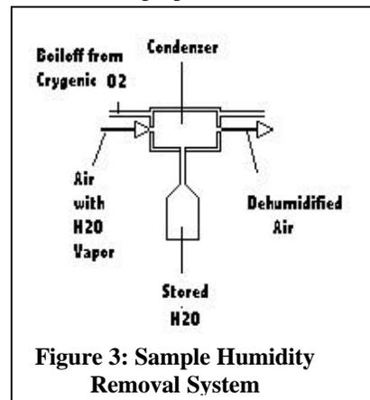
**Figure 3: Sample Humidity Removal System**
