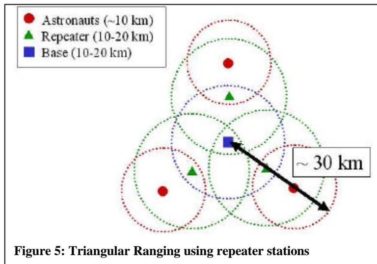
**Figure 5: Triangular Ranging using repeater stations**
