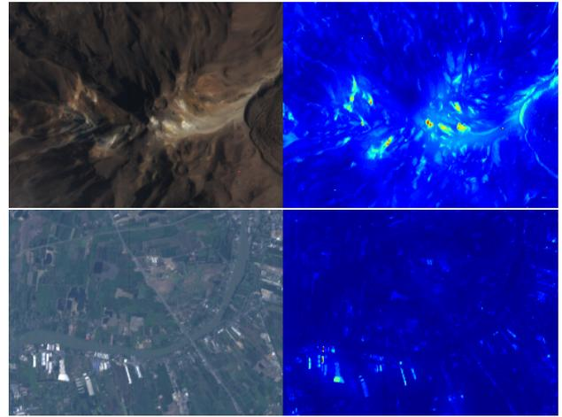
Figure 2: EO-1 onboard novelty detection for a volcano in Chile (top) and buildings in Thailand (bottom): RGB (left) and saliency heat map (right).
